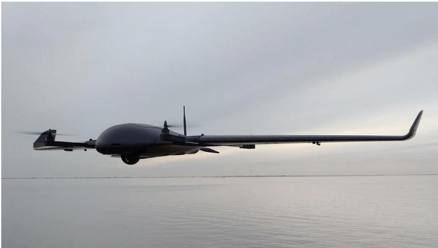
**Figure 2: Drone VTOL DeltaQuad Pro with flight distance - 150 km and single charge flight - 160 min.**
