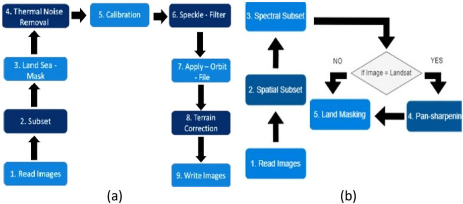
**Figure 2: Workflow of the image dataset preprocessing (a) SAR, (b) optical imagery.**
