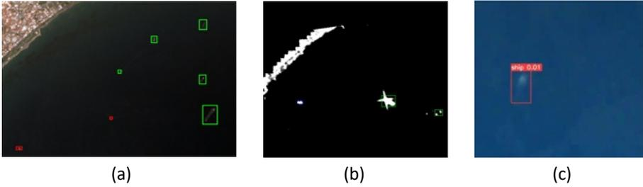
**Figure 9: Application of vessel detection algorithm on (a) Sentinel-2 image, (b) Sentinel 1 image, (c) NEMO HD video.**
